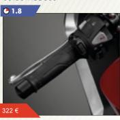
Slim-profile heated grips featuring integrated control with three settings, 'smart' heat allocation that focuses on the hand area most cold-sensitive and battery-drain protection. Quartet harness (08A70-MGS-D30) and heated grips attachment (08T70-MJL-D10) are required to fit this accessory. Special heat-resistant glue (08CRD-HGC-20GMA) is also available.
