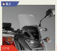
50mm taller and 40mm wider fly screen provides improved wind protection.
